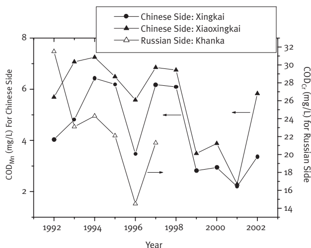
Figure 4. Annual Average Chemical Oxygen Demand (COD) Concentration (mg/L) (Source: Derived from UNEP 2001, p. 30 with additional data provided by author).
